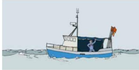
Vessel with reasonable freeboard
